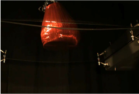
canopy test / tempered glass / 50 kg (110 lb)
